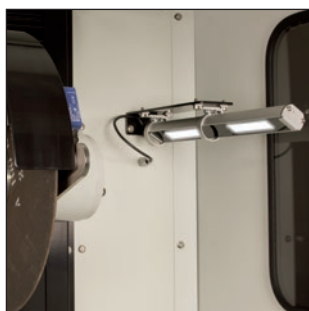
The work area is lit by a LED spotlight.
